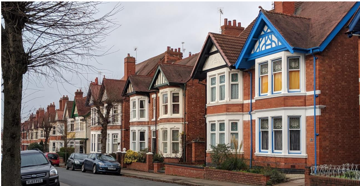
Fig 3.21. Spencer Avenue is characterised by a significant rhythm of red brick and roughcast render semi-detached dwellings, enhanced by street trees and long range views to the landscaping of Spencer Park. The road incorporates examples of historic tiling to doorways and pathways, characteristic stone detailing around bay windows, and a strong rhythm of gable ends incorporating half-timbering. Despite a high level of surviving detailing, there are some examples where this timberwork has been replaced with uPVC panelling, and there has been general rebuilding of historic boundary treatments.
